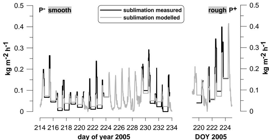
**Fig. 3.** Sublimation rates during the measuring series at the SEBS for  $P^-$  (left) and  $P^+$  (right). The model values (grey) were obtained by taking  $z_m=2.0\text{ mm}$  and  $z_s=1.0\text{ mm}$  for  $P^-$  and  $z_m=20\text{ mm}$  and  $z_s=10\text{ mm}$  for  $P^+$ . They are averaged in correspondence with the temporal resolution of the measurements.
