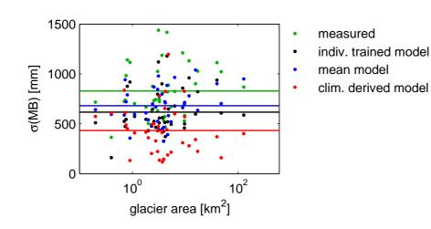
**Fig. 5.** Standard deviation of the annual mass balance plotted against the area of the glaciers. Green dots show  $MB_{measured}$ , black dots show the values of the individually trained model, blue dots show the results of the mean model, and red dots show the results of the climatologically derived model. Horizontal lines show the respective means.
