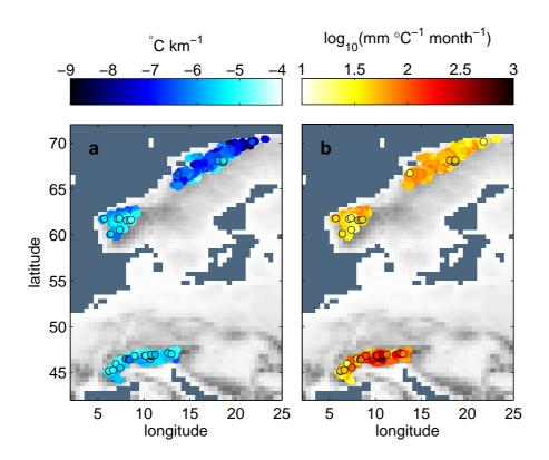
**Fig. 2.** Maps of the model parameters of the climatologically derived model: (a) temperature lapse rates. Values where the correlation between temperature and elevation is below the 95% confidence interval have been omitted. (b)  $\mu_{clim}$ . Markers with black circle indicate the results of the glaciers with more than 12 existing measurements of annual mass balance. Gray background shading: Topography of the CRU TS 3.0 data.
