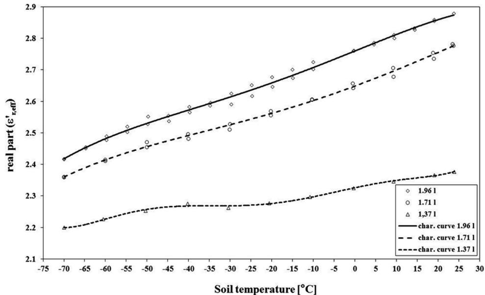
**Fig. 11.** Temperature dependence of  $\epsilon'_{r,\text{eff}}$  for JSC Mars 1 at 350 kHz for 1.37, 1.71, and 1.96 monolayers of water (l) in the range from  $-70$  to  $25$  °C.
