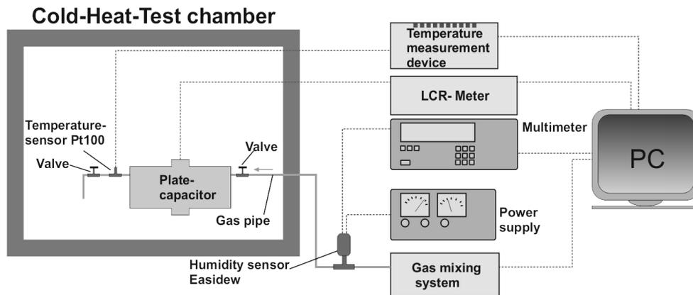
**Fig. 3.** Measurement system.
