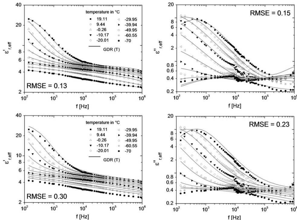
**Fig. 7.** Complex effective permittivity of the clay sample in case of a constant water content of 1.53 monolayers water measured in the temperature range from  $-70\text{ }^{\circ}\text{C}$  to  $20\text{ }^{\circ}\text{C}$  parameterized with the GDR (top) at each temperature and (bottom) in combination with Eqs. (6) or (12) simultaneously.
