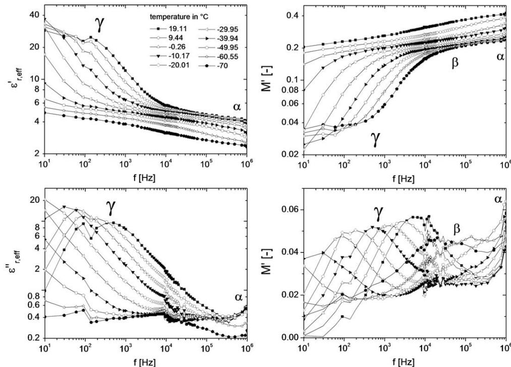
**Fig. 4a.** (Top) real part and (bottom) imaginary part of the complex effective permittivity  $\epsilon_{r,eff}^*$  or complex modulus  $M^* = 1/\epsilon_{r,eff}^*$  of the clay sample in case of a constant water content of 1.53 monolayers water measured in the temperature range from  $-70$  to  $20^\circ\text{C}$ .
