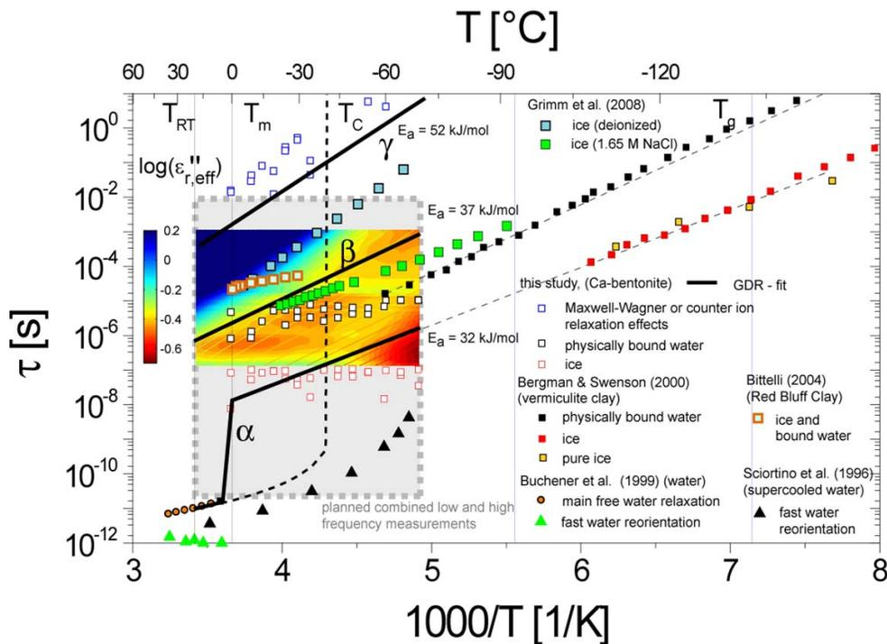
**Fig. 9.** Relaxation map of the Ca-Bentonite (1.53 water monolayers) in comparison to results from aqueous solution with different electrolyte concentrations, ice, as well as clay soils. The contour-plot represents the measured imaginary part of the relative complex effective permittivity.
