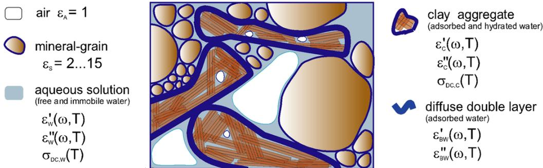
**Fig. 1.** Simplified schematic illustration of the structure of an unsaturated soil sample indicated are the contributions of the single components to the dielectric material properties in terms of a complex effective relative permittivity  $\epsilon_{r,eff}^* = \epsilon'_{r,eff} - j \cdot \epsilon''_{r,eff}$  with real  $\epsilon'_{r,eff}$  and imaginary part  $\epsilon''_{r,eff}$  (cf. Wagner and Scheuermann, 2009).
