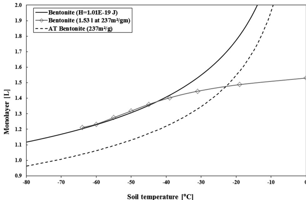
**Fig. 15.** Interfacial water content of the clay soil based on the sandwich-model (black solid line), the deduced values of the 1.53 L line from Table 5 (gray line) and the Anderson–Tice equation (20) (dotted line).
