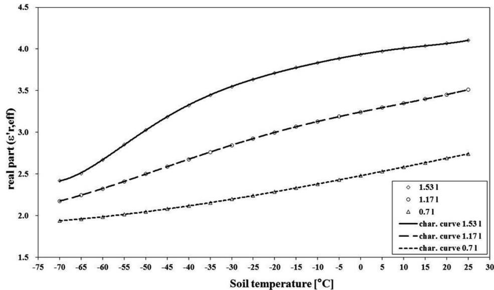
**Fig. 10.** Dependence of  $\varepsilon'_{r,\text{eff}}$  for the clay soil at 350 kHz for 0.7, 1.17 and 1.53 monolayers water (l) in a temperature range from  $-70$  to  $25$  °C.
