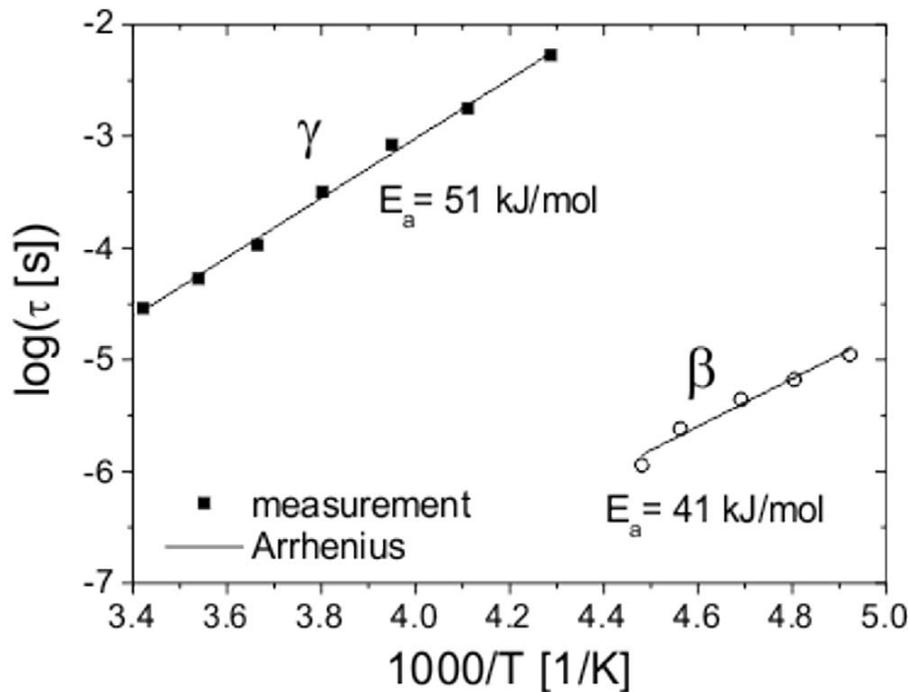
**Fig. 5.** Arrhenius representation of the relaxation time  $\tau = f_{\max}^{-1}$  for the two processes  $\beta, \gamma$  obtained from the appropriate maximum frequency  $f_{\max}$ .
