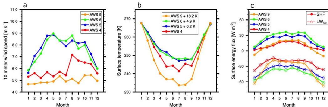
**Fig. 2.** Monthly mean (a) 10 m wind speed ( $V_{10m}$ ), (b) surface temperature ( $T_s$ ) and (c) sensible heat flux (SHF) and net longwave radiation ( $LW_{net}$ ) for AWS 4, AWS 5, AWS 6 and AWS 9. The temperature curves for AWS 5, 6 and 9 (Fig. 2b) are shifted upward by 0.2, 4.9 and 18.2 K respectively, to correct for elevation and continentality differences (Van den Broeke, 2004).
