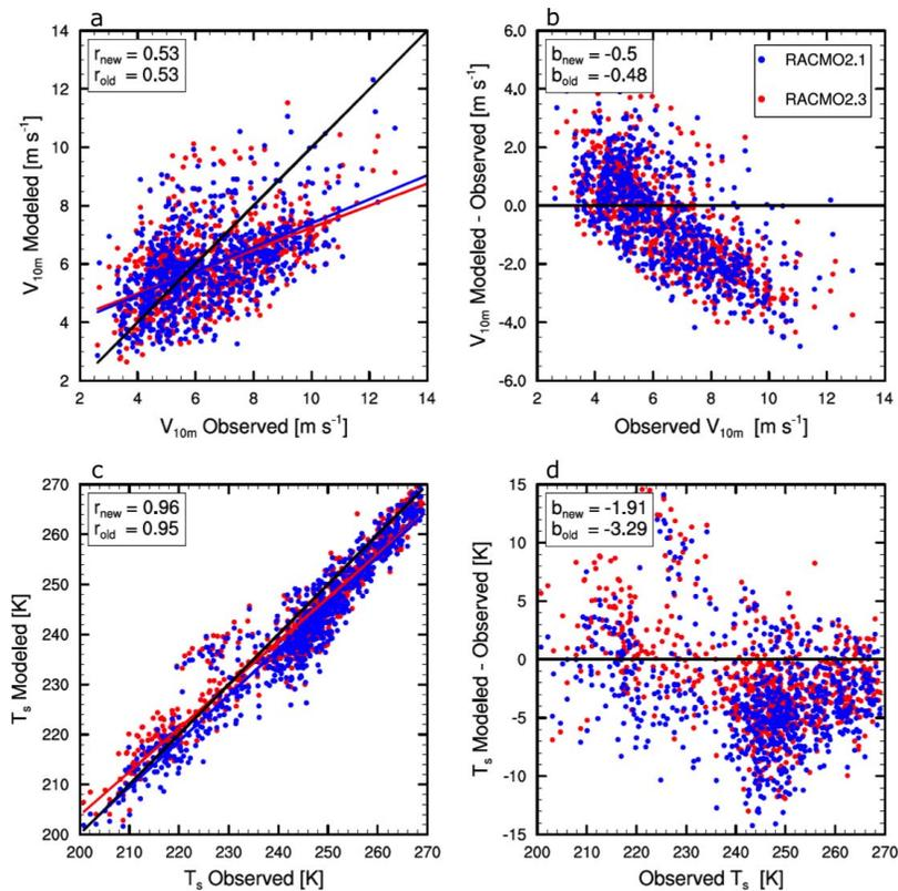
**Fig. 3.** Modelled and difference (modelled – observed) as a function of the AWS observations of **(a, b)** monthly averaged 10 m wind speed ( $V_{10m}$ ) and **(c, d)** surface temperature ( $T_s$ ). Shown are RACMO2.3 (red) with correlation  $r_{new}$  and bias  $b_{new}$  and RACMO2.1 (blue) with correlation  $r_{old}$  and bias  $b_{old}$ . Biases are averages over all data with units [ $m s^{-1}$ ] for  $V_{10m}$  and [K] for  $T_s$ .
