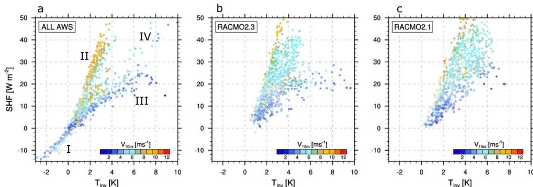
**Fig. 11.** Monthly averaged SHF as a function of the surface temperature inversion ( $T_{inv} = T_{2m} - T_s$ ) for **(a)** all AWSs, **(b)** RACMO2.3 and **(c)** RACMO2.1. The color scheme represents wind speed  $V_{10m}$  and model data is from the same months and locations as the observational data. Filled circles are winter values (months 4–9) and open circles represent months (10–3).
