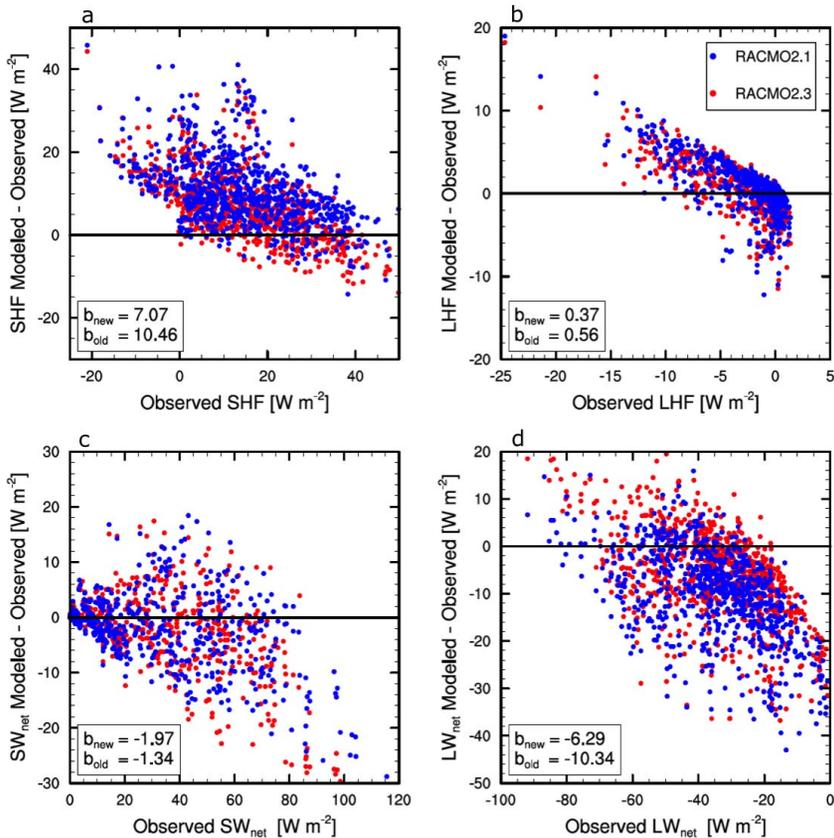
**Fig. 5.** Difference (modelled – observed) of **(a)** sensible heat flux (SHF), **(b)** latent heat flux (LHF), **(c)** net shortwave radiation ( $\text{SW}_{\text{net}}$ ) and **(d)** net longwave radiation ( $\text{LW}_{\text{net}}$ ) as a function of the AWS observations. Shown are RACMO2.3 (red) with bias  $b_{\text{new}}$  and RACMO2.1 (blue) with bias  $b_{\text{old}}$ . Biases (in  $[\text{W m}^{-2}]$ ) are averages over all monthly average weather station data ( $> 750$  data points).
