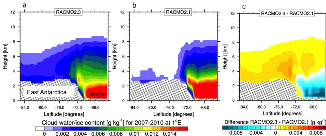
**Fig. 10.** Latitudinal cross-section of yearly (2007–2010) averaged total cloud water/ice content for (a) RACMO2.3, (b) RACMO2.1 and (c) the difference (RACMO2.3 – RACMO2.1) at 1°E. Location of cross-section is indicated in Fig. 1.
