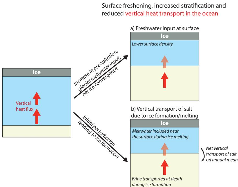
**Fig. 4.** Schematic representation of the stabilization of the Southern Ocean by sea ice processes
