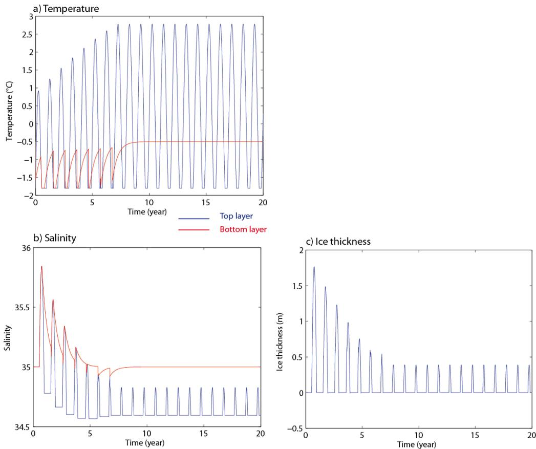
**Fig. 10. (a)** Temperature (K), **(b)** salinity, and **(c)** sea ice thickness (m) in the two-layer model after an instantaneous reduction of the temperature in the surface layer. The value of the top layer is in blue, the bottom one is in red.
