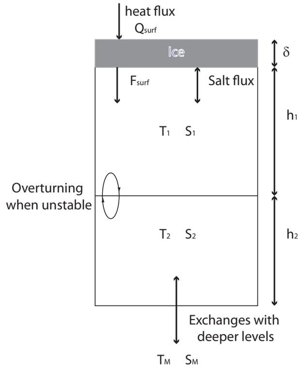
**Fig. 8.** Schematic representation of the two-layer model displaying the dominant processes included and the state variables.
