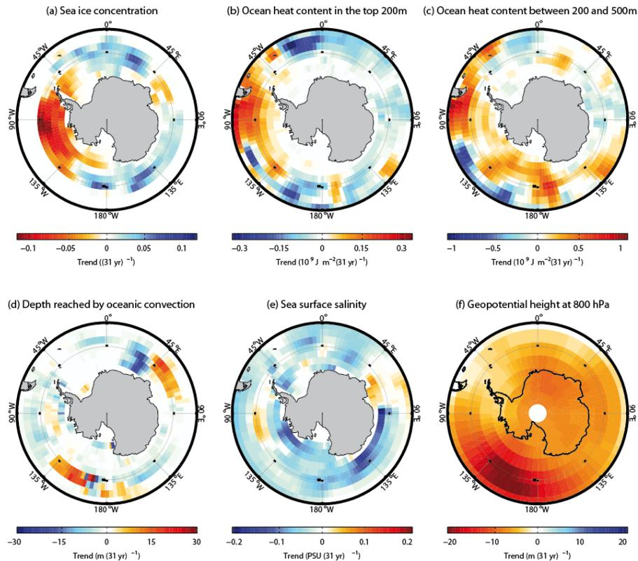
**Fig. 12.** Trends over the period 1979–2009 in a simulation with LOVECLIM using data assimilation scaled to represent the 31 yr changes of **(a)** ice concentration, **(b)** ocean heat content in the top 200 m ( $\text{J m}^{-2}$ ), **(c)** ocean heat content in the layer between 200 and 500 m ( $\text{J m}^{-2}$ ), **(d)** depth reached by oceanic convection (m), **(e)** sea surface salinity, **(f)** geopotential height at 800 hPa (m).
