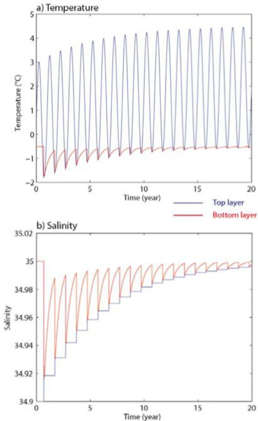
**Fig. 9. (a)** Temperature (K) and **(b)** salinity in an experiment performed with the two-layer model initialized from a weakly stratified state. The value of the top layer is in blue, the bottom one is in red.
