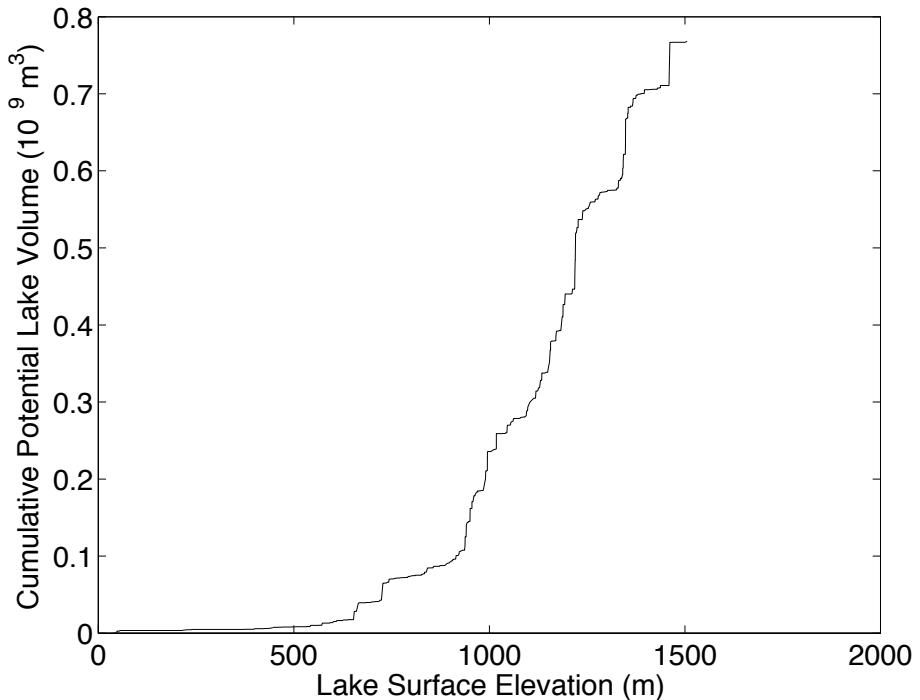
**Fig. 4.** Cumulative maximum potential surface water storage in surface depressions by elevation for the Paakitsoq region.
