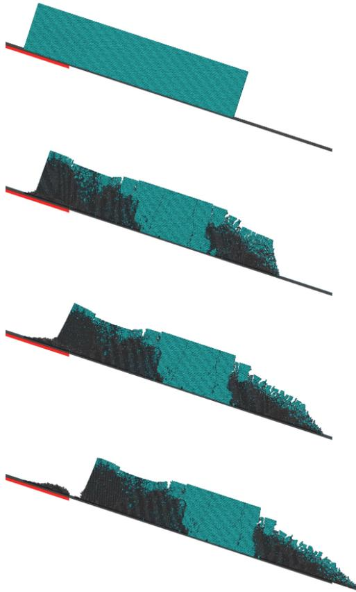
**Fig. 5.** Snapshots of a 200 m × 50 m ice-block on a 18° slope. The red line marks a high friction contact. The colors of the ice-block represent elastic areas where the elastic beams between particles have not been broken (green) and viscous areas where beams are no longer intact (gray). The pressure of upstream ice slab on the slope above the ice-block is not shown in the figure.
