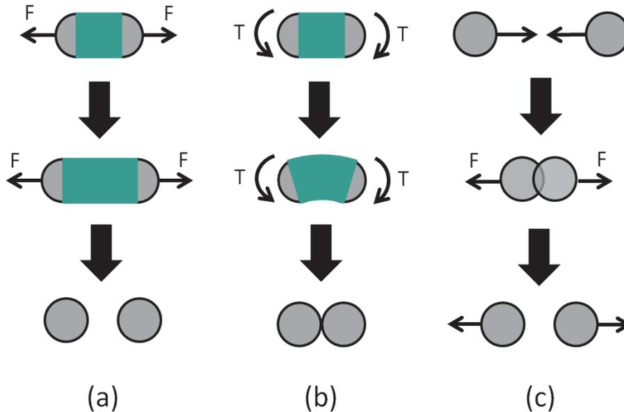
**Fig. 1.** The particles connected with a beam can **(a)** stretch when a force  $F$  is applied and **(b)** bend when a torque  $T$  is applied. Particles that overlap, i.e. come into contact **(c)** will experience repulsive forces. The amount of stretching and bending required for beam breaking is highly exaggerated as is the amount of overlapping of the particles occurring in the simulations.
