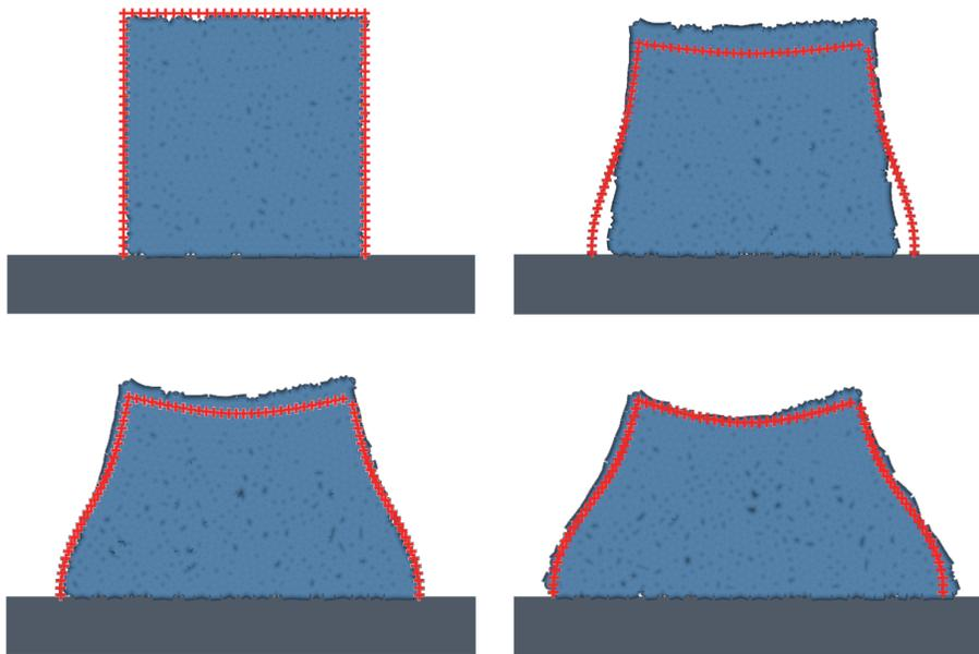
**Fig. 4.** Snapshots of a deforming ice block simulated with Elmer/Ice and our particle model. In the Elmer/Ice simulation (red markers) the snapshots are from timesteps 0, 3, 5 and 7 yr and the particle model snapshots (blue area) are from corresponding time steps. The size of the block is 30 m × 30 m and the time span of the Elmer/Ice simulation is roughly  $10^8$  s compared to the  $10^3$  s time span of the particle simulation.
