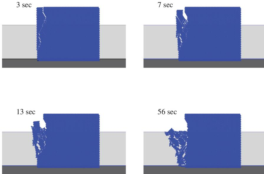
**Fig. 2.** Snapshots of a calving ice-block. The size of the block is 30 m × 30 m. The block rests on a soft substrate that efficiently hinders the block from sliding, thus modelling e.g. a muddy sea floor. The block is immersed in 20 m of water. The simulation times of the snapshots are indicated.
