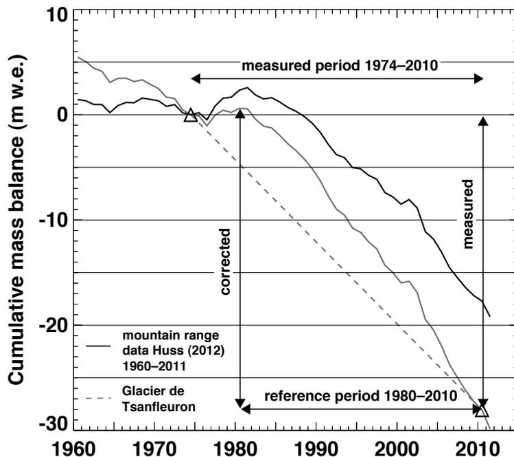
**Figure 3.** Temporal homogenization of cumulative average mass balance from DEM differencing for Glacier de Tsanfleuron (dark grey) based on cumulative mean annual mountain-range mass balance from Huss (2012).
