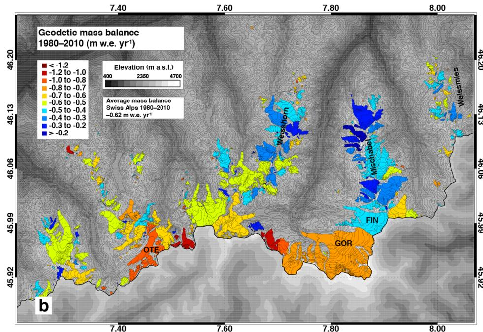
**Figure 9.** Spatial distribution of the temporally homogenized geodetic mass balance 1980–2010 for the central/eastern Valais Alps. The SGI2010 outlines are taken to illustrate glacier surface area.
