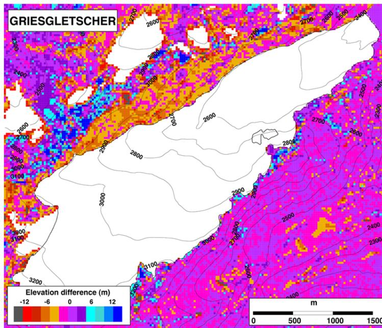
**Figure 4.** Comparison of input DEMs over stable terrain. The 1973 extents of Griesgletscher and adjacent smaller glaciers are masked out.
