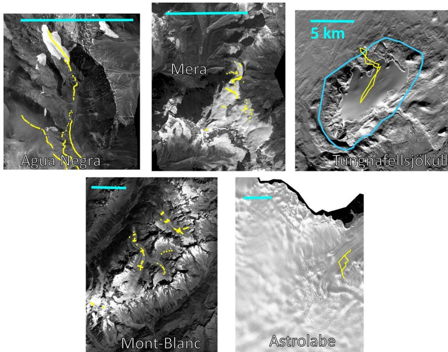
**Figure 2.** Pléiades ortho-images for the 5 different study sites. Yellow dots locate the GNSS measurements used to evaluate the DEMs. For Tunghafellsjökull, the blue polygon marks the limits of the Lidar DEM. The horizontal blue scale bar has a length of 5 km in each panel.
