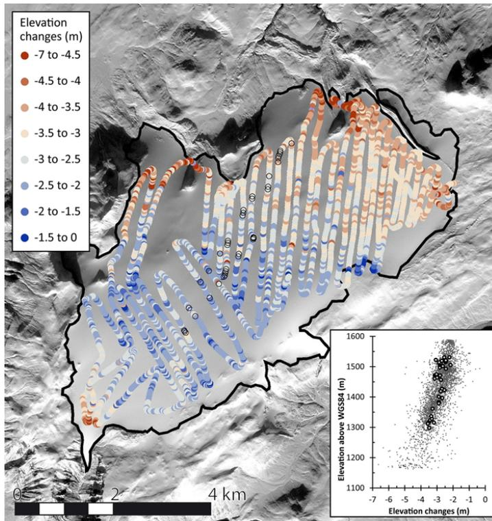
**Figure 4.** Elevation differences between the kinematic GNSS data (2 May 2013) and the Pléiades DEM (9 October 2013) on the Tunngafellsjökull Ice Cap. Black circles indicate the locations where elevation differences have been measured using repeated GNSS surveys (2 May 2013 and 18 September 2013). Inset: distribution of these elevation differences with altitude, with repeat GNSS surveys shown as larger dots. Background: Pléiades image (© CNES 2013, Distribution Airbus D&S).
