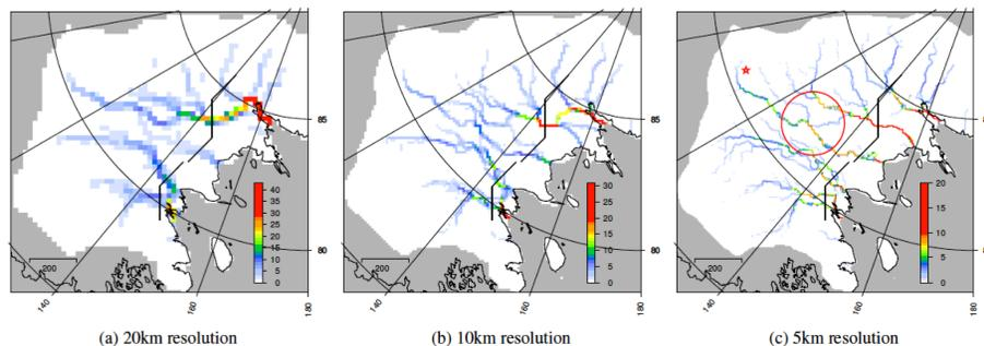
**Figure 2.** Simulated basal water pathways for present-day bedrock elevation and ice thickness. Color scales show the drainage in percent of the total catchment area. Figures show also five defined cross sections, corresponding to the locations of the main trunks of the Ross Ice Streams A–E, Fig. 1) to quantify the associated water drainage. (Red star and circle, see caption of Fig. 3.)
