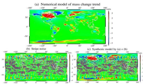
Figure 1. (a) The numerical model of mass change trend, (b) the stripe noise model; (c) synthetic model by (a) + (b).
