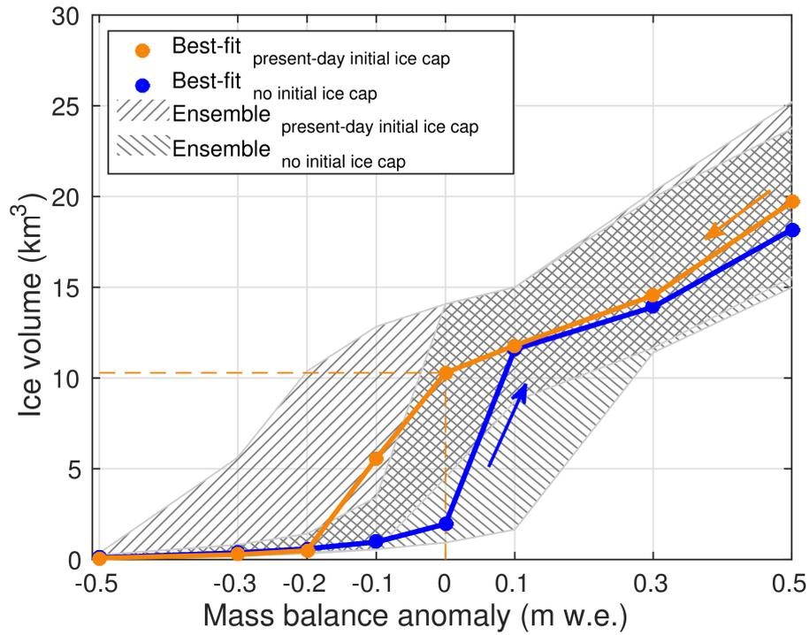
**Figure 10.** Steady-state ice volumes reached using step perturbations of the 1963-2007 mass balance, using an ensemble of dynamical parameter combinations, starting from the present-day ice cap and ice-free conditions.
