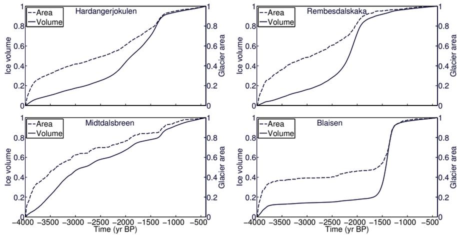
**Figure 12.** Simulated ice volume and area evolution for (a) Hardangerjøkulen, and the outlet glaciers (b) Rembesdalskåka, (c) Midtdalsbreen, and (d) Blåisen, from 4000 to 400 BP (1600 AD). Quantities are non-dimensionalized relative to final volume and area in year 1600 AD, respectively.
