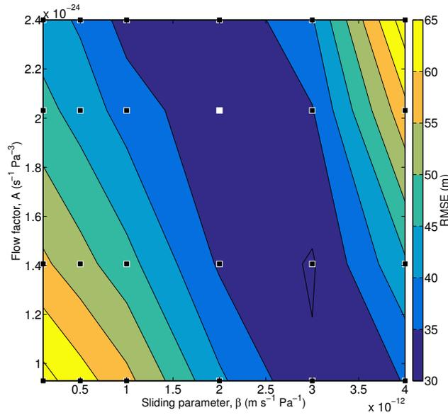
**Figure 3.** Root mean square error (RMSE) between modelled and observed present-day ice thickness along the flowlines of Middtdalsbreen and Rembesdalskåka, using an ensemble of sliding ( $\beta$ ) and rheology ( $A$ ) parameters. Shown are parameter combinations (black squares) and the 'best-fit' parameter combination used in subsequent runs (white square).
