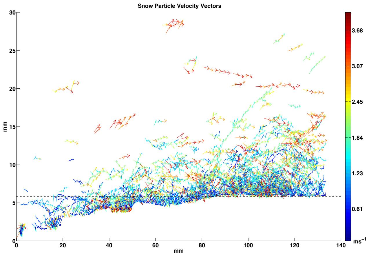
**Figure 2:** Sparse snow particle velocity vector field during one second of recording on 23 March, vector colors scaled according to total particle speed. The dashed line shows reference below which particles are influenced by microtopography.
