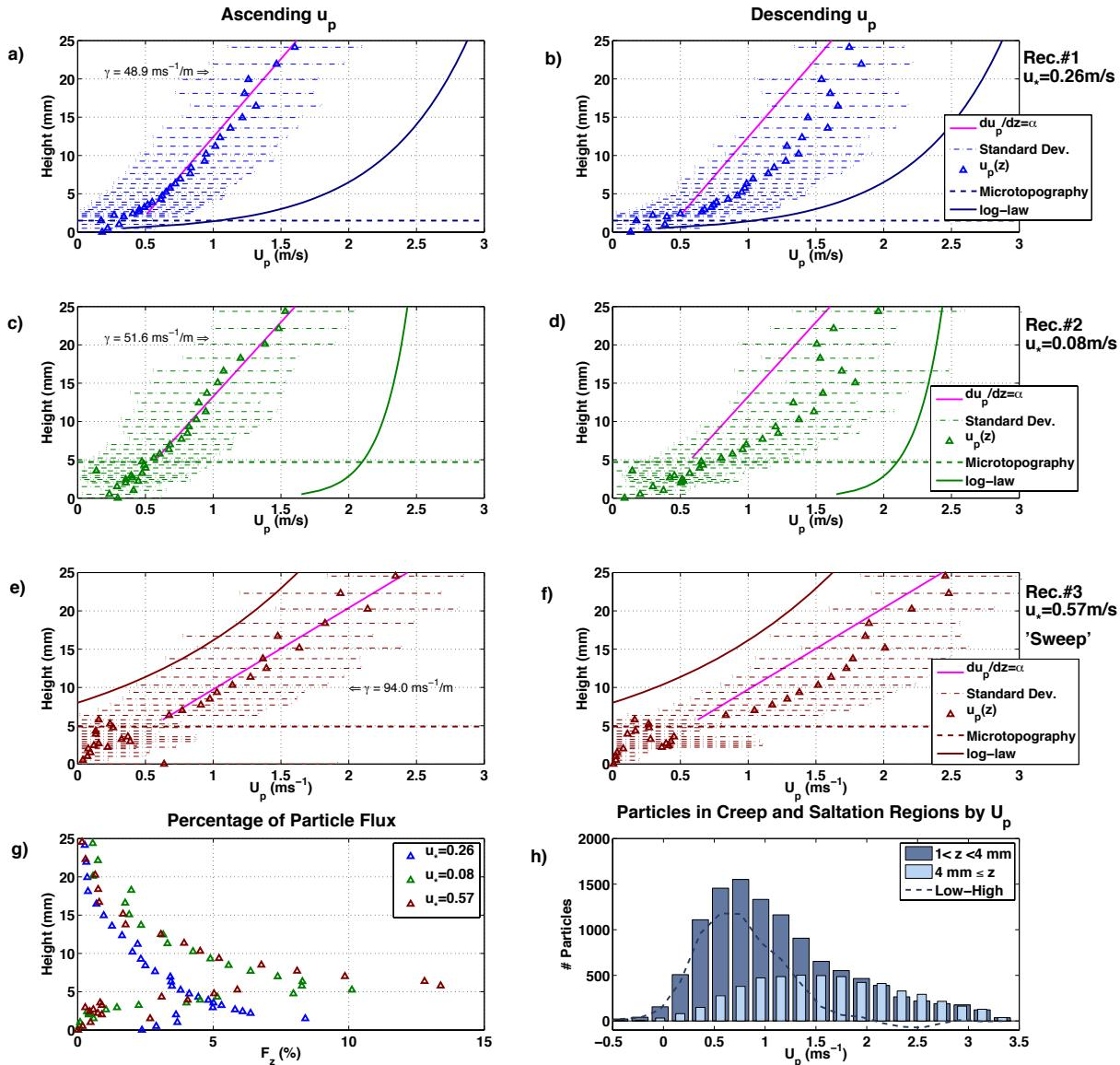
Figure 3 a-f): Ascending and descending mean snow particle horizontal velocity profiles ( $u_p$ ), with one standard deviation error bars, log-law wind profiles for recording specific values (solid lines), and plots of constant  $du_p/dz = \gamma$ . 3g) Particle number flux concentration profiles, 3h) Descending snow particle velocity histograms for two height bands for the  $u_* = 0.57 \text{ ms}^{-1}$  recording on March 23, 2015.
