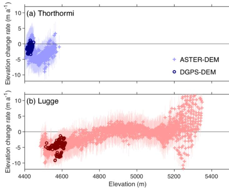
**Figure R11:** Rate of elevation change along elevation at (a) Thorthormi and (b) Lugge Glaciers. Dark-colored circles are from DGPS-DEM and light-colored crosses are from ASTER-DEM. Error bars denote standard deviations of DEM differences over the ice-free terrain.
