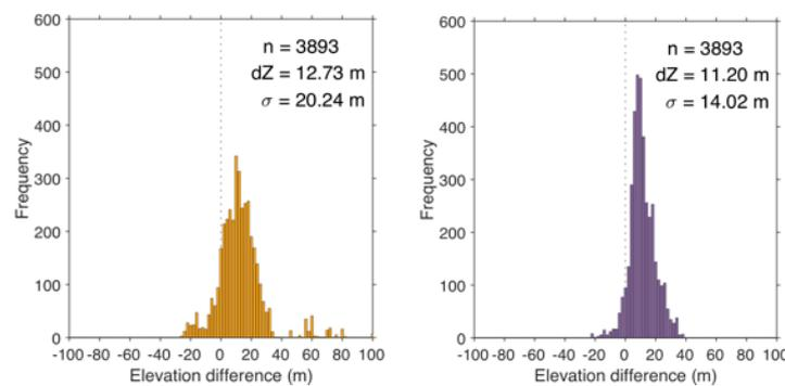
**Figure R9:** Elevation differences in the ice-free area (left) between 2004 ASTER-DEM and DGPS-DEM and (right) between 2011 ASTER-DEM and DGPS-DEM.
