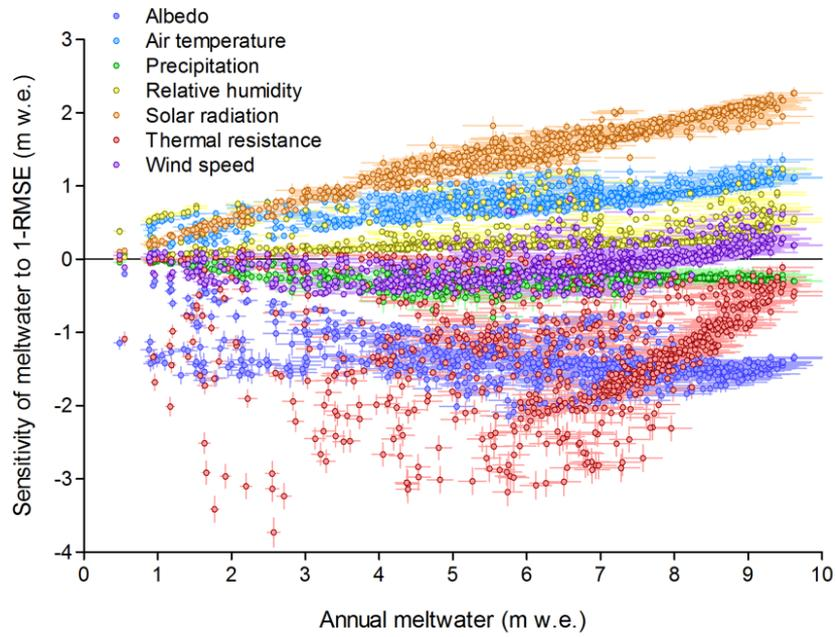
**Figure R6:** Sensitivity analysis of annual meltwater at debris-covered area as a function of variation of each parameter. RMSEs of ERA-Interim against the observed data were used for the meteorological variables. Uncertainty derived from 8 satellite images are used for thermal resistance and albedo.
