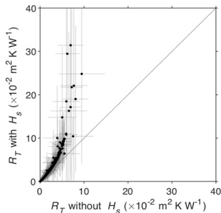
**Figure R4:** Scatter plot between thermal resistance calculated from only net radiation (without  $H_s$ ) and from net radiation + sensible heat (with  $H_s$ ).
