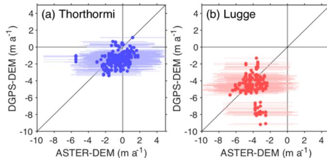
**Figure R10:** Scatter plot of the rate of surface elevation change between from ASTER-DEMs and DGPS-DEMs at (a) Thorthormi and (b) Lugge Glaciers. Error bars denote standard deviations of DEM differences over the ice-free terrain.
