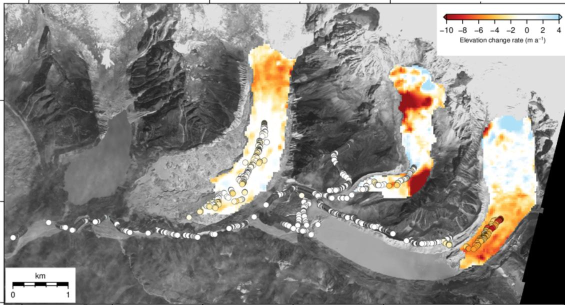
**Figure R1:** Rate of elevation change for the 2004–2011 period derived from ASTER-DEMs (background shadings) and DGPS-DEMs (circles filled with the same color scale). Glacier outlines are of December 2011.
