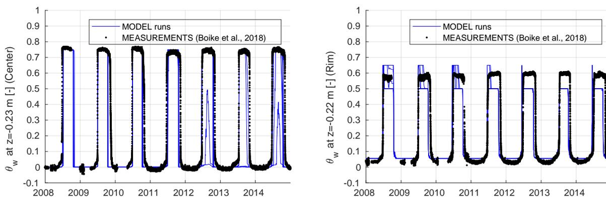
**Figure E2.** Modelled versus measured soil moisture levels for a polygon centre (left) at a depth of 0.23 m and for a rim (right) at a depth of 0.22 m, for 2008 to 2014. Measurement data from Boike et al. (2018). Model results are for all validation runs (see Table 4, VALIDATION).
