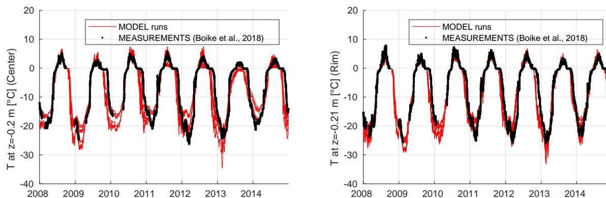
**Figure E1.** Modelled versus measured soil temperatures for a polygon centre (left) at a depth of 0.20 m and a polygon rim (right) at a depth of 0.21 m, for 2008 to 2014. Measurement data from Boike et al. (2018). Model results are for all validation runs (see Table 4, VALIDATION).
