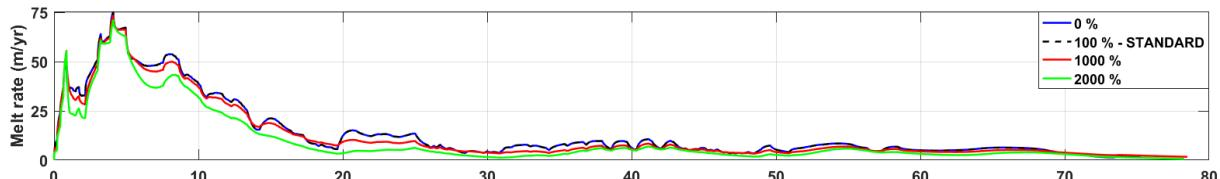
**Figure S5:** Sensitivity of the submarine melt rate along the centreline of the 79NG ice tongue due to the tidal flow in the cavity. The tidal velocity in the STANDARD case is 1.18 cm/s. Note that this are results from Anhaus, 2017 (Master thesis, unpublished) and here the STANDARD case has tides of 1.18 cm/s and a subglacial discharge of  $1 \times 10^{-3} \text{ m}^2/\text{s}$ .
