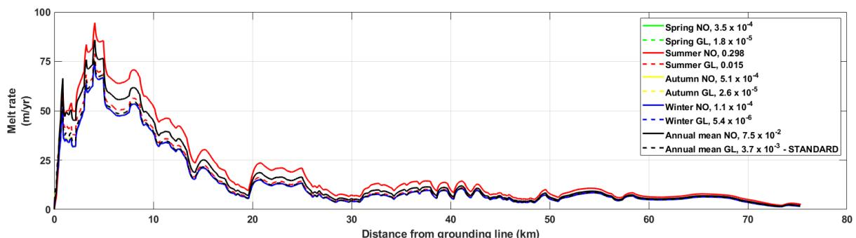
**Figure S4: Sensitivity of the submarine melt rate along the centreline of the 79NG ice tongue due to the seasonality and distribution of subglacial discharge ranging from  $5.4 \times 10^{-6} \text{ m}^2/\text{s}$  (winter, GL) to  $0.298 \text{ m}^2/\text{s}$  (summer, NO).**
