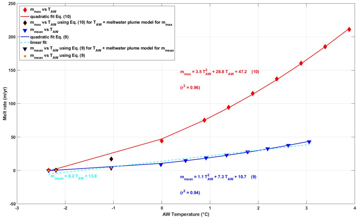
**Figure 5. Mean melt rate along the centreline of the 79NG ice tongue (blue), maximum melt rate in the grounding line zone (red), and melt rate calculated using the quadratic fit function (green) depending on the AW temperature as described in the text.**
