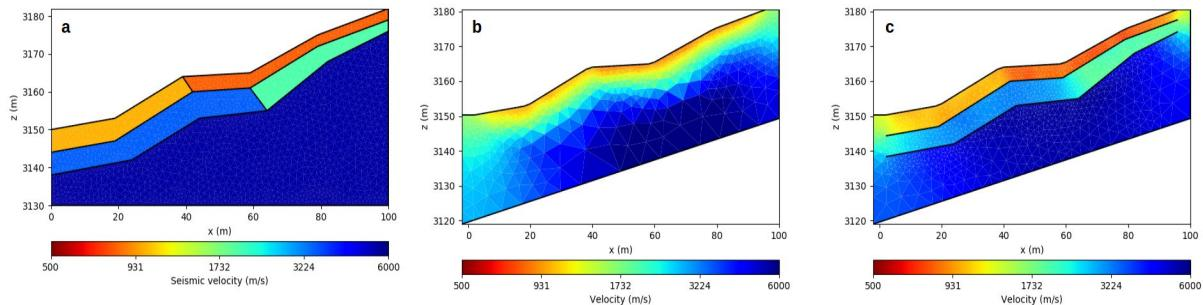
**Figure R2: Synthetic model a proposed in Figure R1 (left-hand plot) and the obtained inversion results using smoothness-constrained inversions (b) and after the incorporation of structural constraints (c)**
