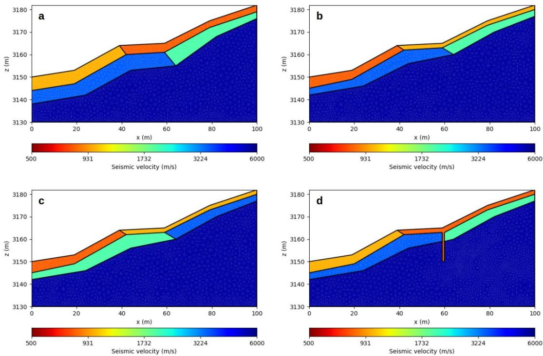
**Figure R1: Proposed models for the revised version of our manuscript associated to: dipping layers, variable thickness and lateral velocities changes, fractures.**
